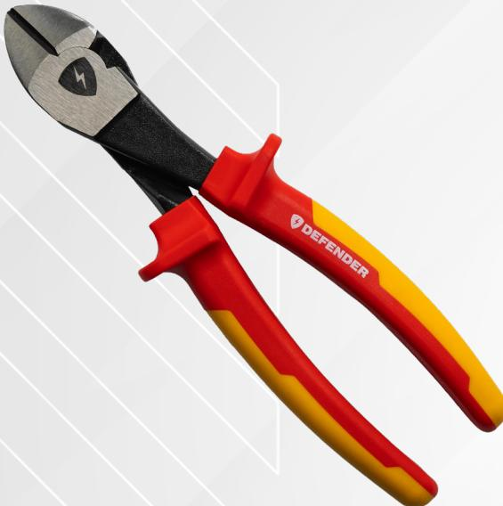
These 8-inch insulated diagonal cutters are VDE certified and guaranteed for safe use in electrical environments up to 1000V. Designed to meet the IEC 60900 standard for safe work near live parts. Made of CR-MO steel with a hardness level of 58 HRC (Rockwell scale). Built with strength and durability, these pliers can cut through hard wire up to 4.2mm thick and 2.5mm piano wire. For use in -40°F to 158°F temperatures. Ergonomic rubber grip handle with slip guards.
